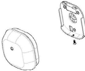
2. Unscrew the screw from the battery cover and remove the battery cover.
