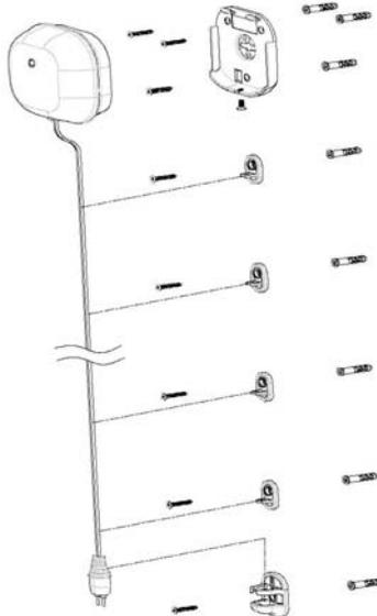
3. Fix the back cover, water sensor cable rack and sensor rack using the fixing screws provided.
