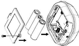
4. Refit the battery cover by fastening its screw.
